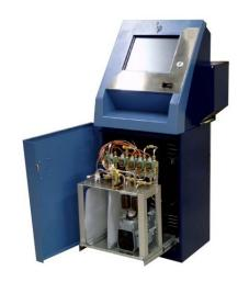
Radiation Monitoring Equipment – Software, Control System, ion chambers designed and manufactured by Tyne
